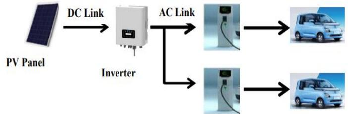
Figure 1: Solar Power EV charging Station diagram
