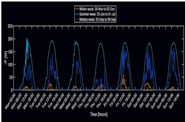
**Figure 3: PV Panel Production graph showing peak, median, and minimum weekly output**
