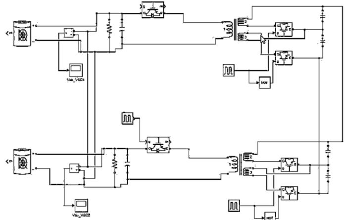
**Figure 2: Battery charging using bidirectional control**
