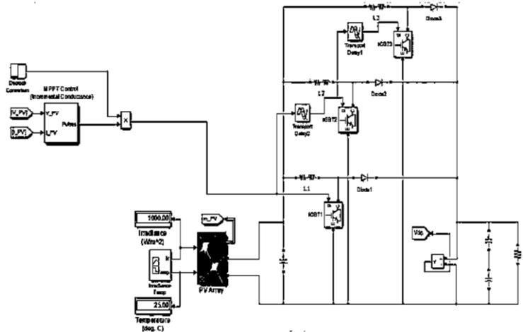
**Figure 1: PV to EV Charging subsystem using MPPT**
